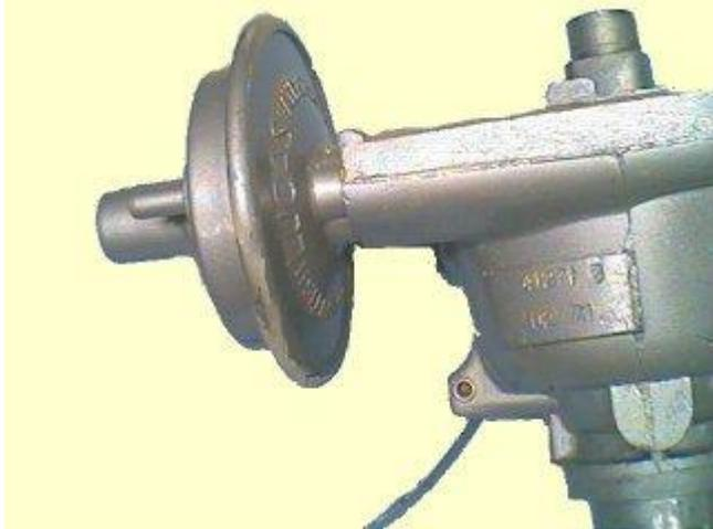
The illustrations above show the 25D distributor. While it remained basically the same there were some variations, particularly in the design of the vacuum advance assembly. Some had screw-on metal tube fittings, some push-on rubber attachments.
