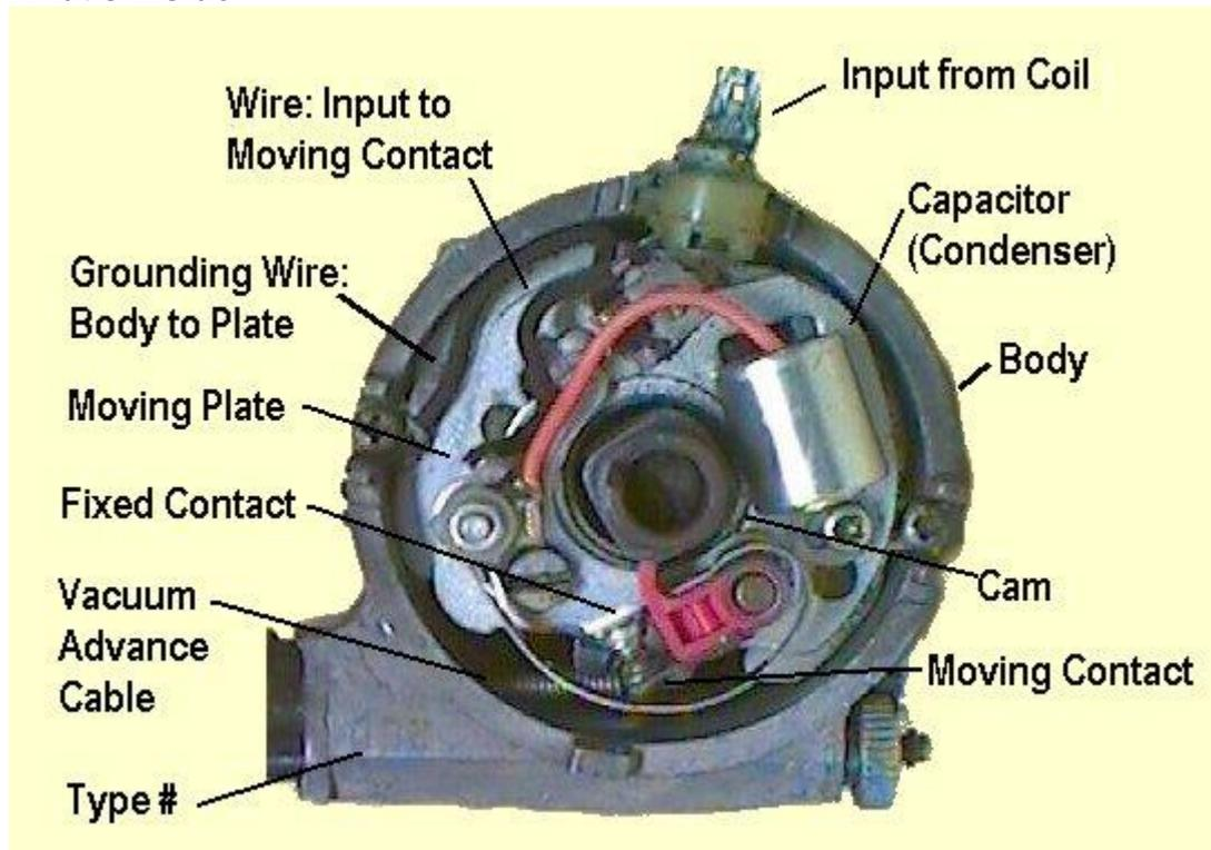
The photo at left shows the Lucas 25D distributor that was fitted to MGA's and MGB's until 1974 and which is typical of many of its era. With the ignition ON, voltage is applied to
