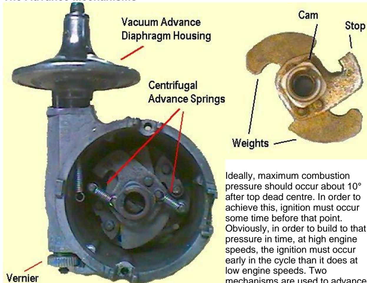
Ideally, maximum combustion pressure should occur about 10° after top dead centre. In order to achieve this, ignition must occur some time before that point. Obviously, in order to build to that pressure in time, at high engine speeds, the ignition must occur early in the cycle than it does at low engine speeds. Two mechanisms are used to advance
