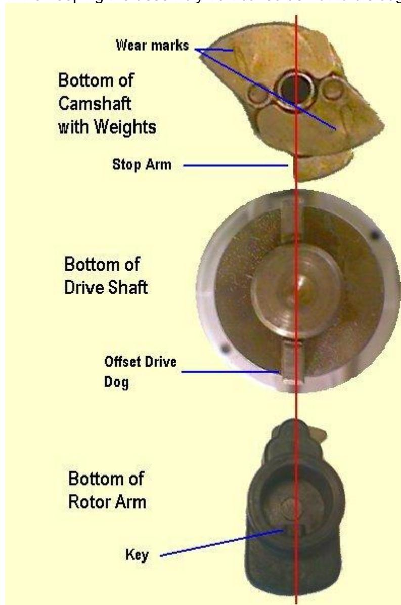
home, the camshaft should seat in the body with the minimum of wiggling.
