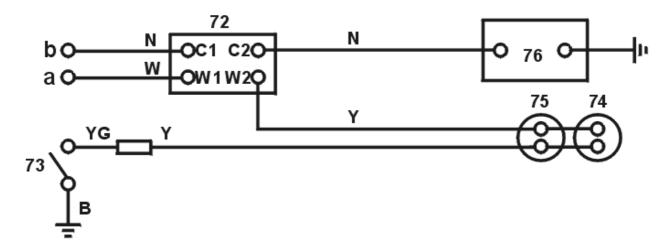
Another interesting fact is that Triumph used a left hand switch for left hand drive cars where you shift with the right hand, and a right hand switch for RHD cars where you shift with the left hand. I' m not making this up. When installing overdrive, use a right hand switch in a LHD car because it' sergonomically correct and the left hand switch blocks the wiper switches in TR4A and TR6 when overdrive is not engaged.
